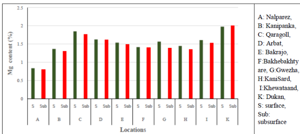
Figure 4: Total concentration of magnesium (Mg) in surface and subsurface samples at the studied locations.
